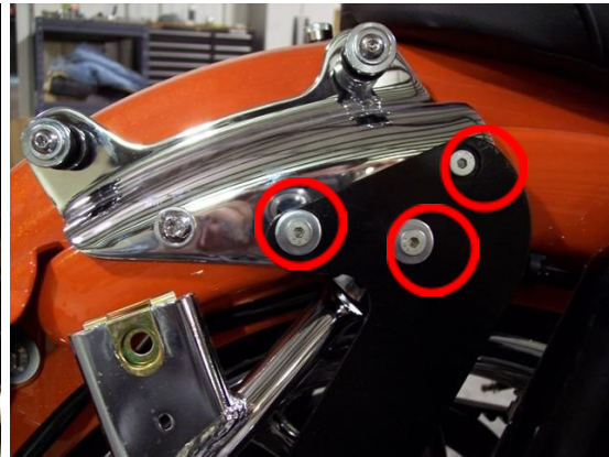
Step 8- Bolt Positions Seen on Right Side of Motorcycle- Rearmost Bolt Position not used for hitch Installation Highlighted
