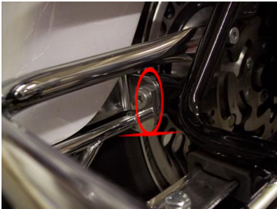
Step 5- Bolt connecting Lower Saddlebag Support to Rear Fender Support Plate highlighted
