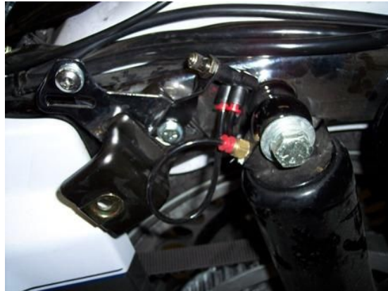
Step 15 & 19- Installation of Schrader Valve with Relocation Bracket
