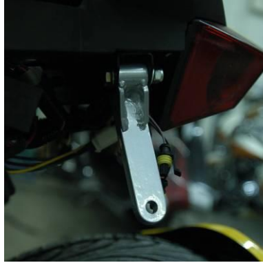
Step 6-Upper Strut Mount-left side shown.
